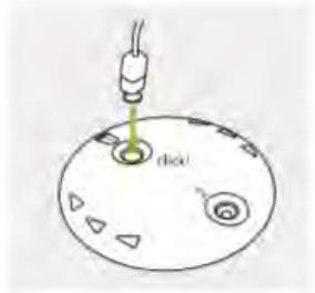
To remove a used wax filter, carefully insert the speaker/wire into the opening under the trash bin icon until it clicks. Remove the speaker and you should see the old wax filter in the opening.
