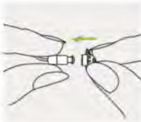
Hold the speaker in one hand and the dome in the other. Slide the dome over the speaker.
