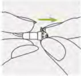
Remove the dome from the speaker by holding the speaker in one hand and the dome in the other. Gently pull off the dome to remove.
